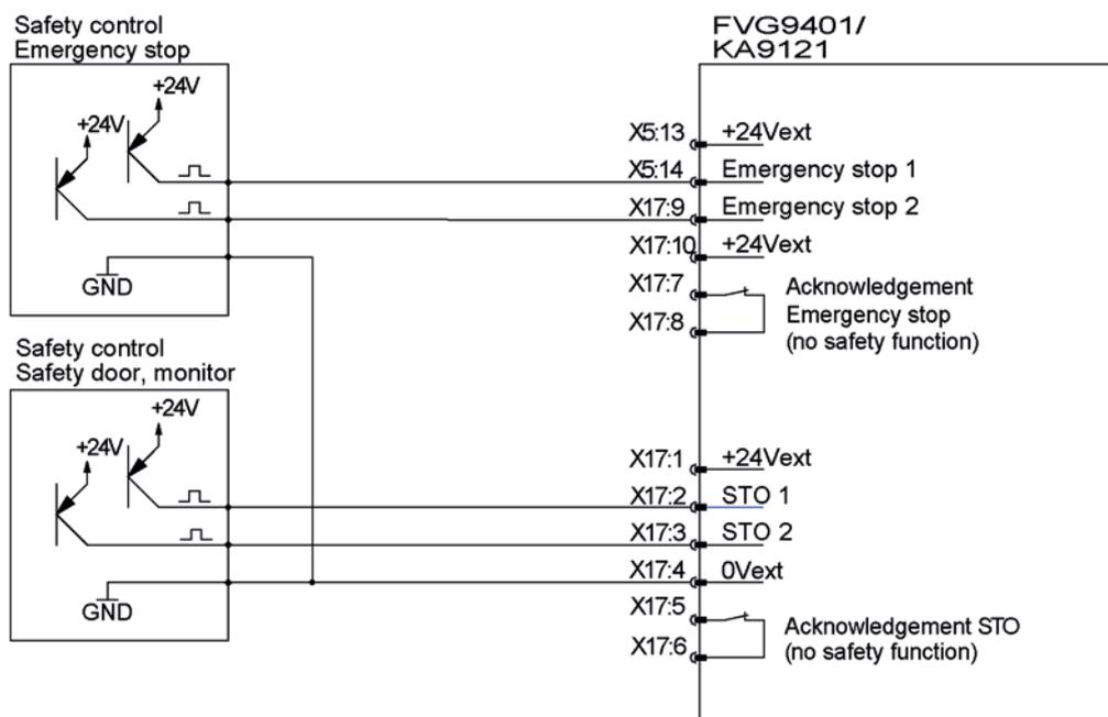
**Attention:** The configuration of X17 has been changed compared to older devices. In case the option SLS is not existing X15 must not be wired.
