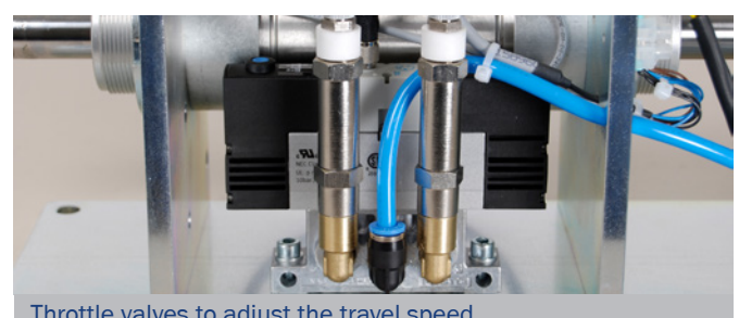
Throttle valves to adjust the travel speed
